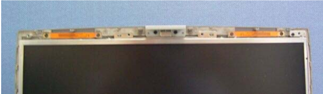
Picture of Antenna installed in the notebook
