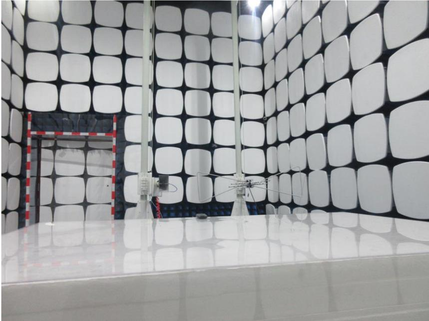
1.4 Radiated Emissions Test Setup
