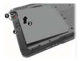
Fit another battery pack into place. With the battery pack correctly oriented, attach its connector side to the battery compartment at an angle (1) and then press down the other side (2). The battery release latch should automatically engage.
