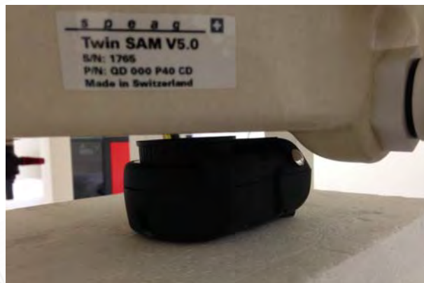
Fig.3 Front side to flat phantom
