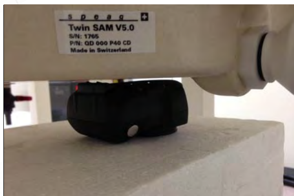
Fig.4 Back side to flat phantom
