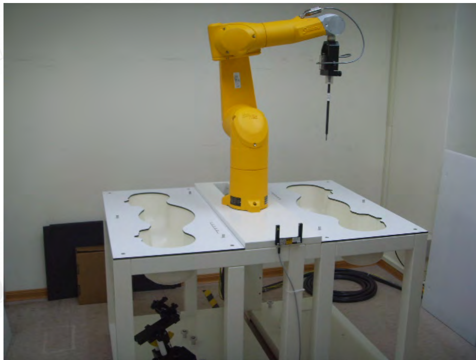
Fig.1 Photograph of the SAR measurement system
