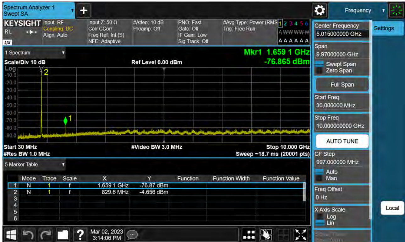
Sub6 n5. Conducted Spurious Plot (167300ch_15 MHz_BPSK_RB 1_1)
