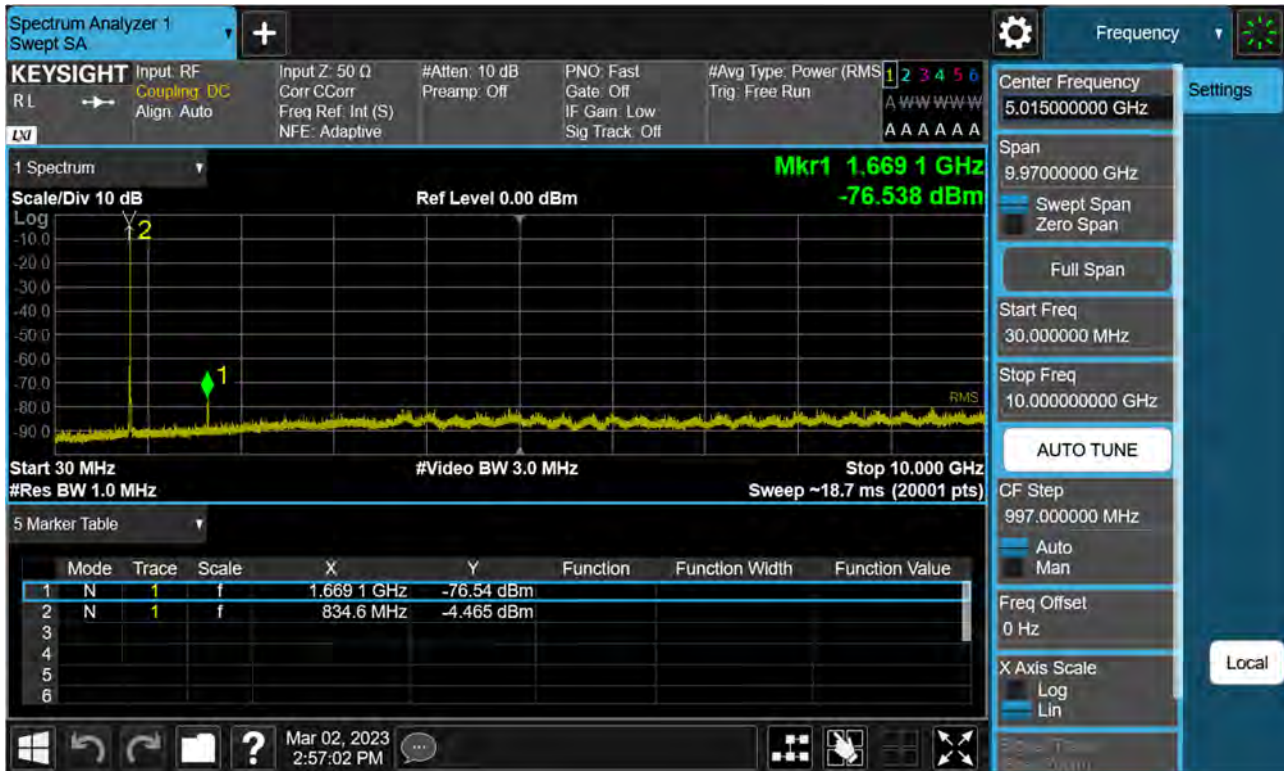
Sub6 n5. Conducted Spurious Plot (167300ch_5 MHz_BPSK_RB 1_1)
