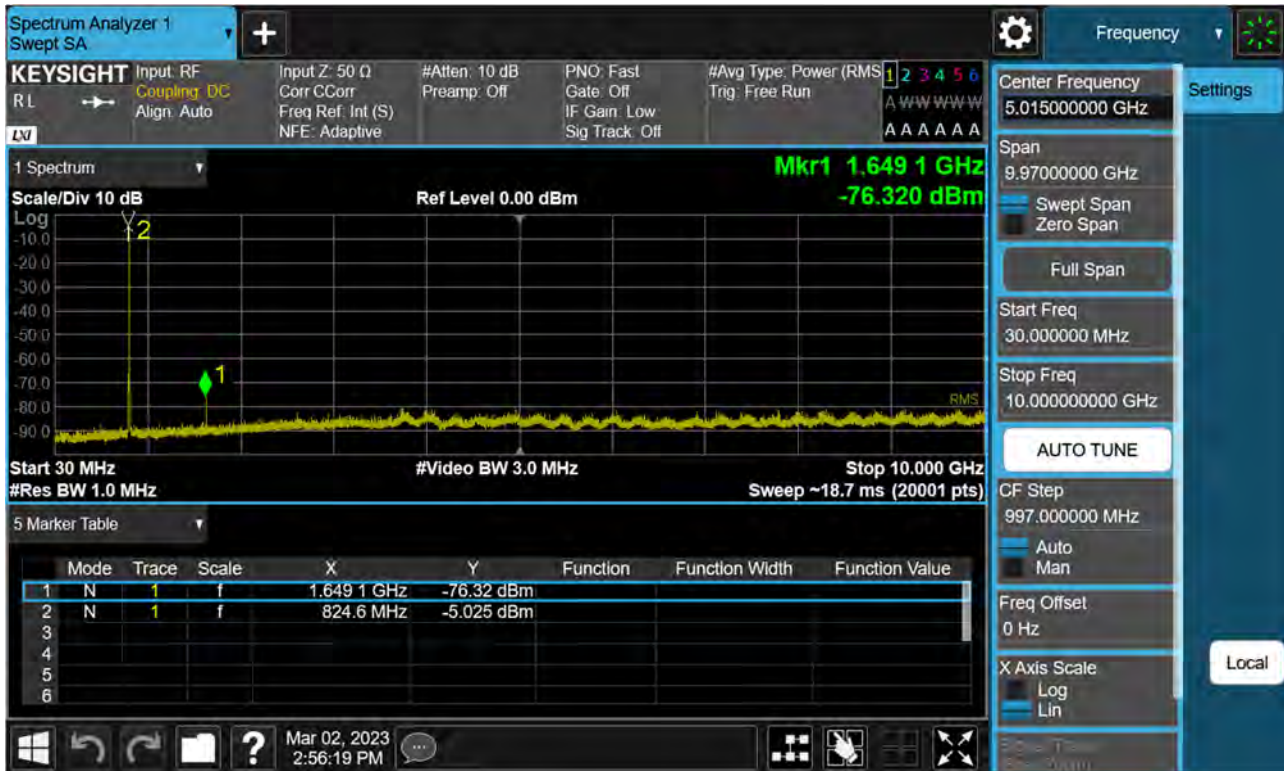
Sub6 n5. Conducted Spurious Plot (165300ch_5 MHz_BPSK_RB 1_1)
