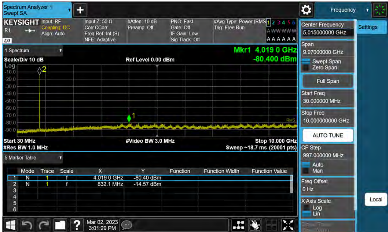
Sub6 n5. Conducted Spurious Plot (167300ch_10 MHz_BPSK_RB 1_1)
