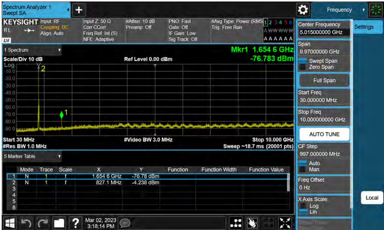
Sub6 n5. Conducted Spurious Plot (167300ch_20 MHz_BPSK_RB 1_1)
