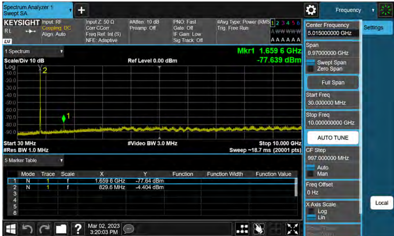
Sub6 n5. Conducted Spurious Plot (167800ch_20 MHz_BPSK_RB 1_1)
