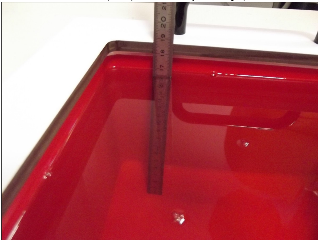
Photo 1: Liquid depth 450 MHz body simulating liquid
