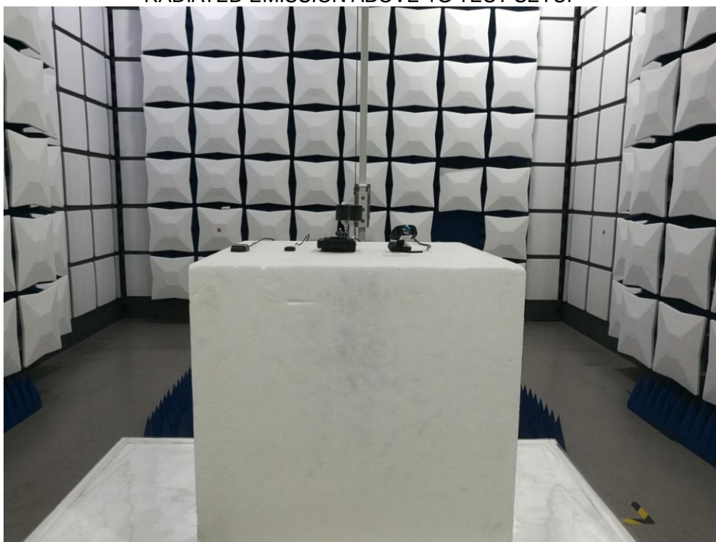
RADIATED EMISSION ABOVE 1G TEST SETUP
