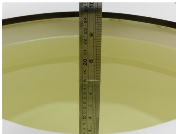
Fig 10.1 Photo of Liquid Height for Body SAR
