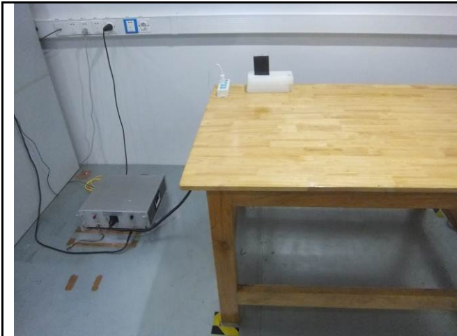
Conducted Emissions Test Setup Front View
