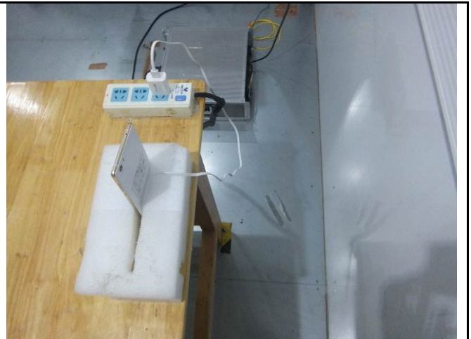
Conducted Emissions Test Setup Side View
