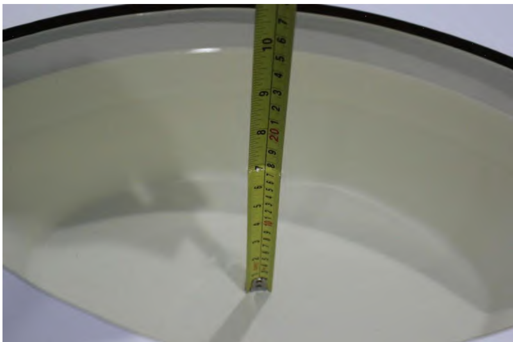
Picture 7-2: Liquid depth in the Flat Phantom(5GHz)
