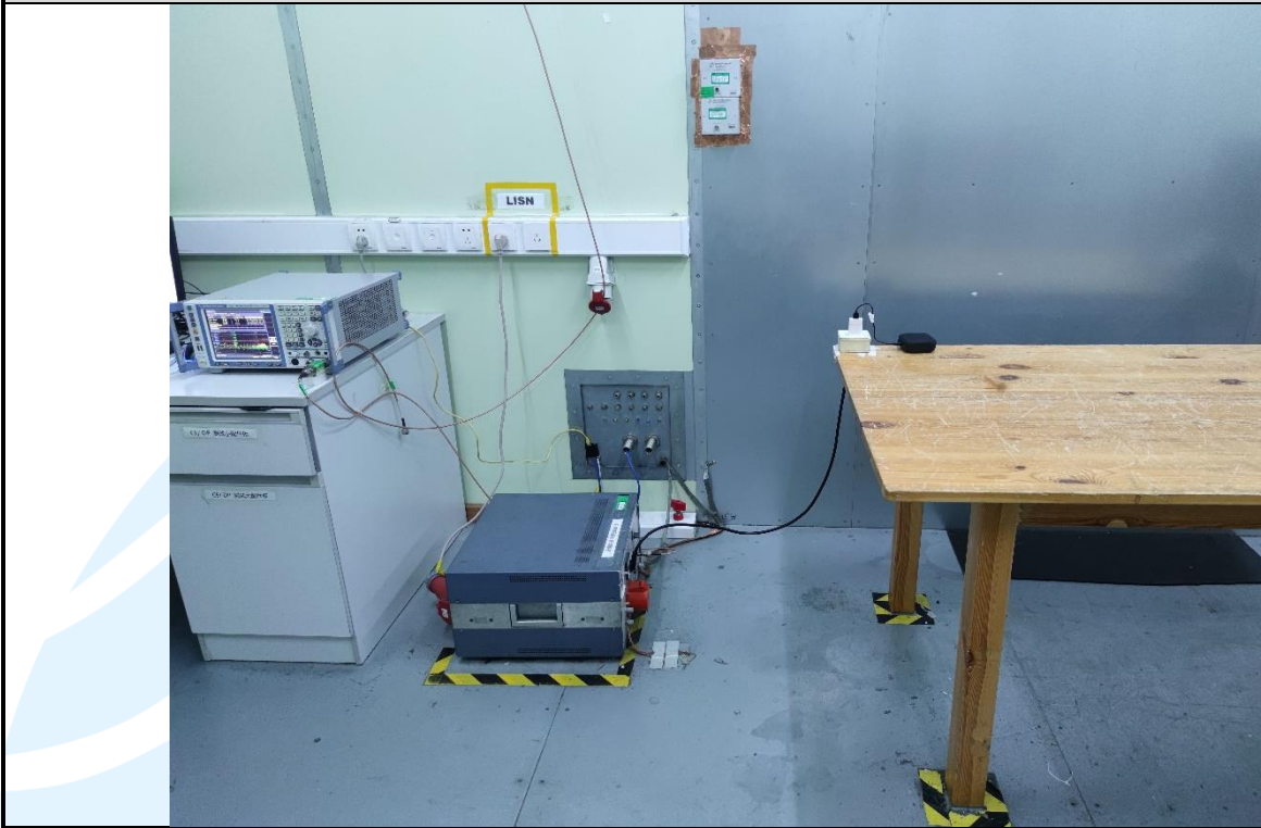
AC Power Line Conducted Emission Test Setup
