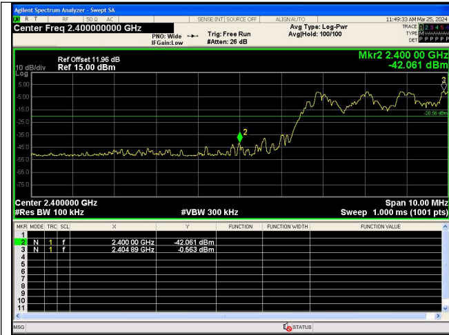
Out Of Band Emission(Left) 8DPSK_3-DH5_Channel Hopping
