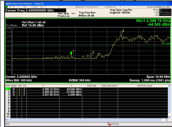
Out Of Band Emission(Left) 8DPSK_3-DH5_Channel Hopping
