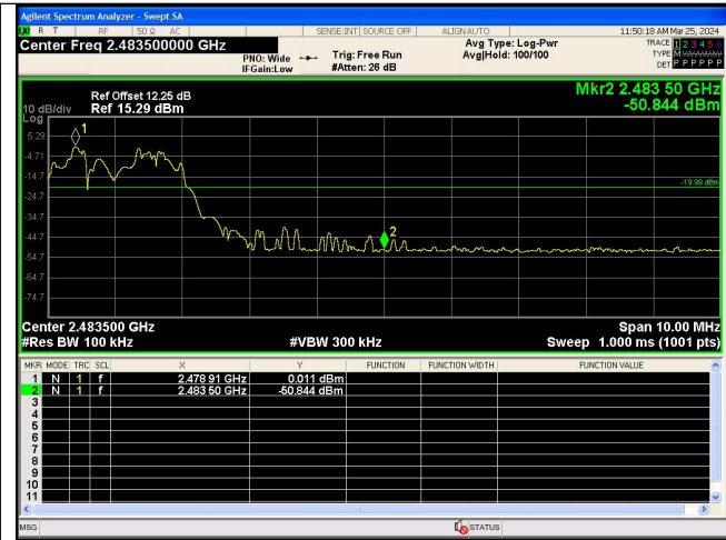
Out Of Band Emission(Right) 8DPSK_3-DH5_Channel Hopping
