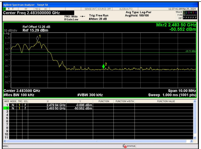
Out Of Band Emission(Right) 8DPSK_3-DH5_Channel Hopping
