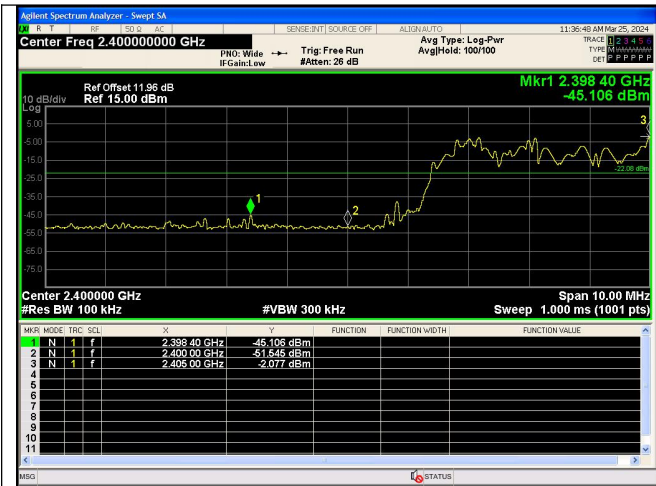
Out Of Band Emission(Left) 8DPSK_3-DH5_Channel Hopping
