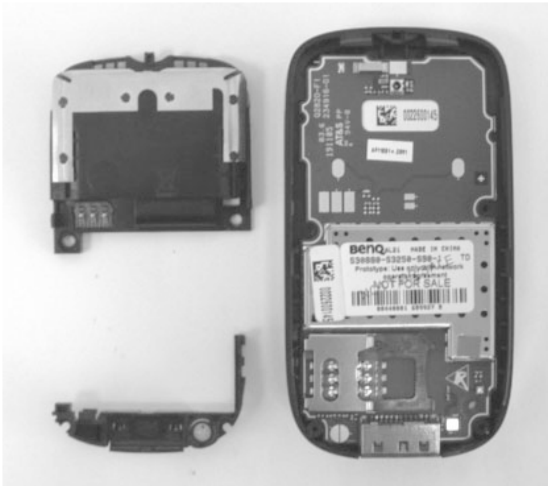
AL21 Disassembly Step 1
