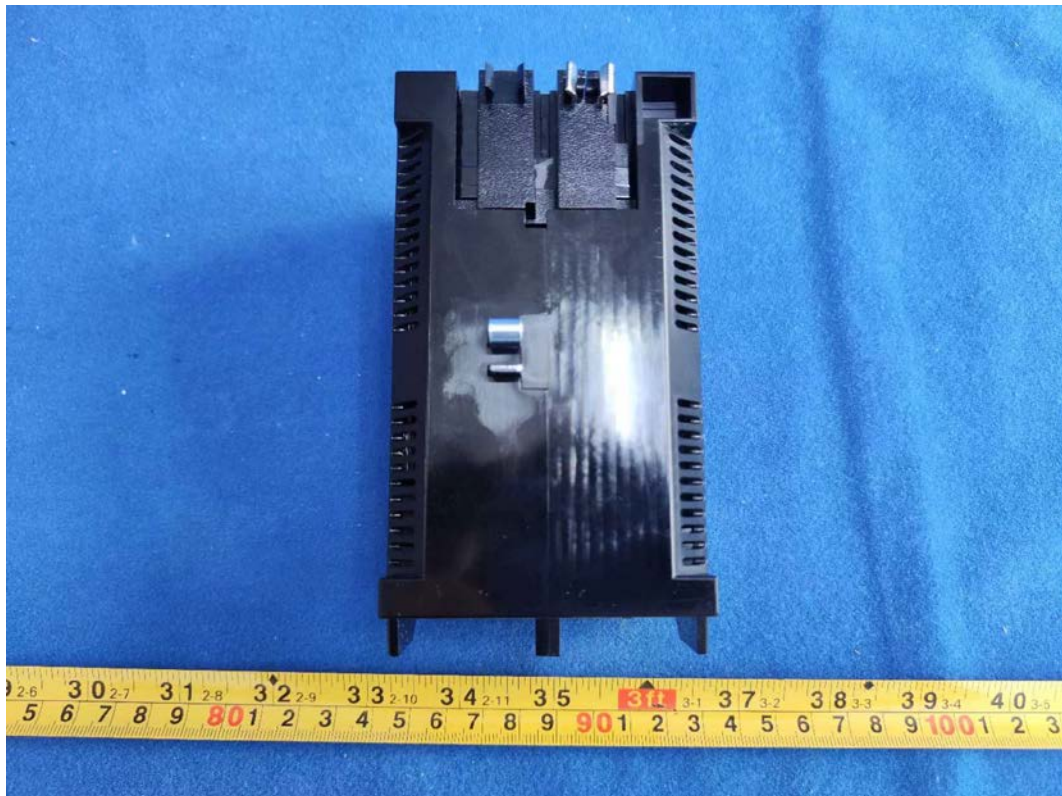
FIGURE 2 240 VAC 60 A WISER CONTROL RELAY (QO260PWX240) BACK APPEARANCE
