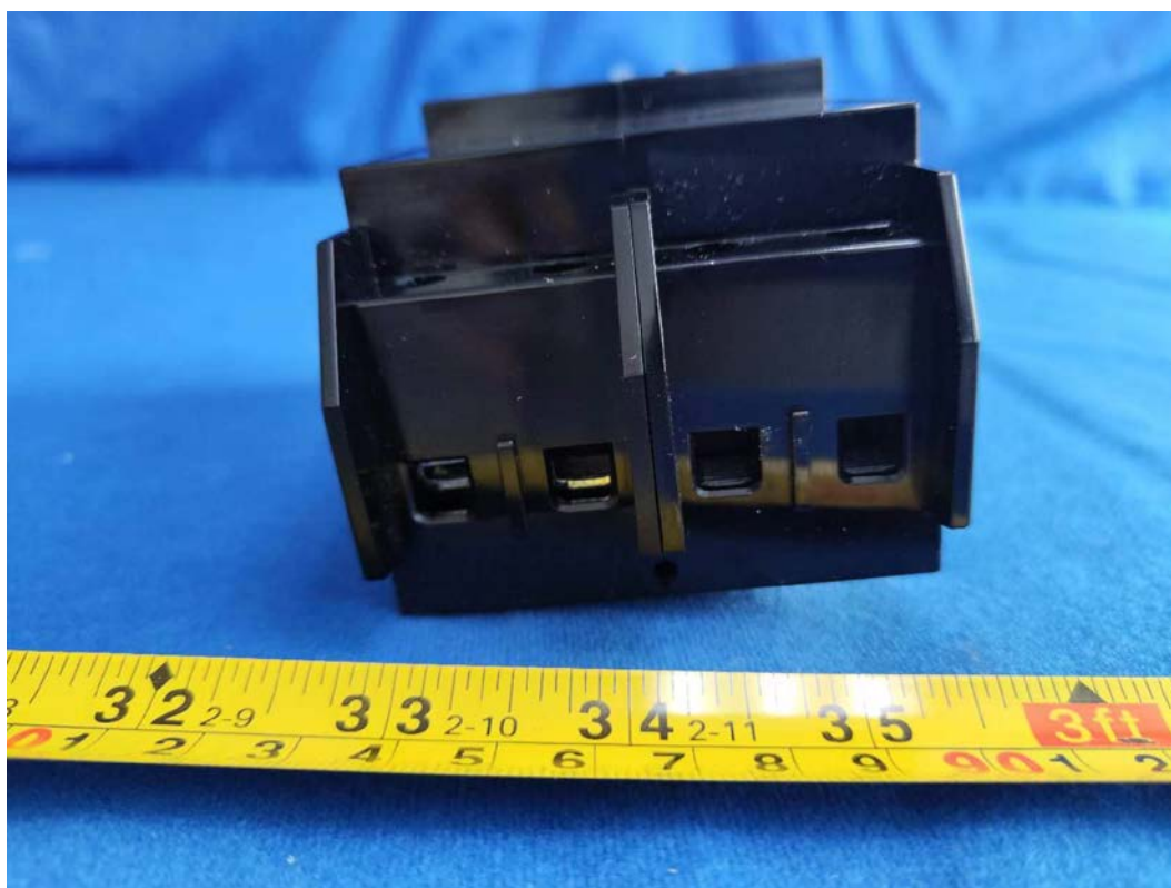
FIGURE 6 240 VAC 60 A WISER CONTROL RELAY (QO260PWX240) BOTTOM
