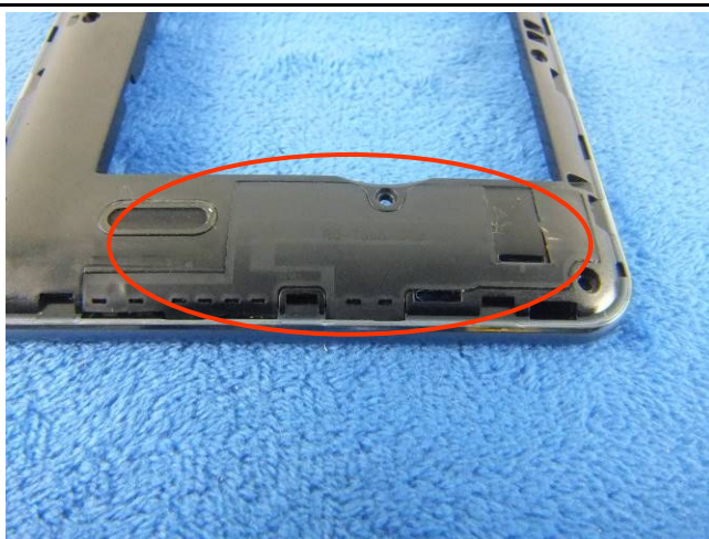
GSM/PCS/UMTS-FDD Antenna View
