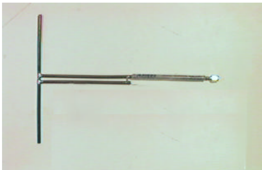
Reference Dipole Antenna Used for ERP Measurement
