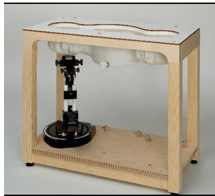
Picture C.10: SAM Twin Phantom
