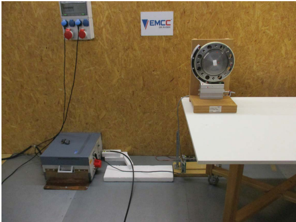
Photo A1-1: Conducted emissions measurement, 150 kHz – 30 MHz
