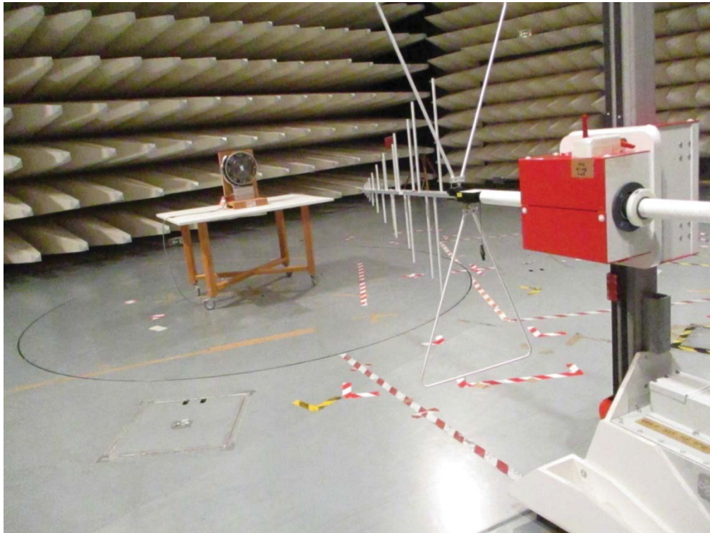
Photo A1-3: Radiated emissions measurement at 3 m distance, 30 MHz – 150 MHz
