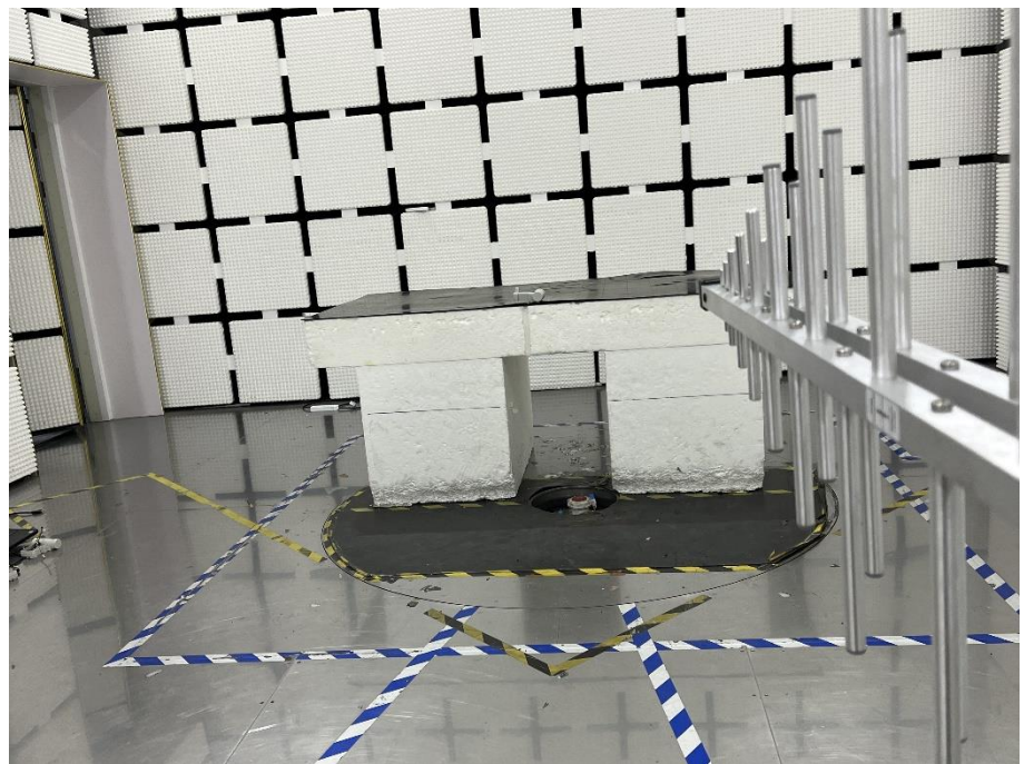
Radiation Emission Test Setup (30MHz to 1GHz)
