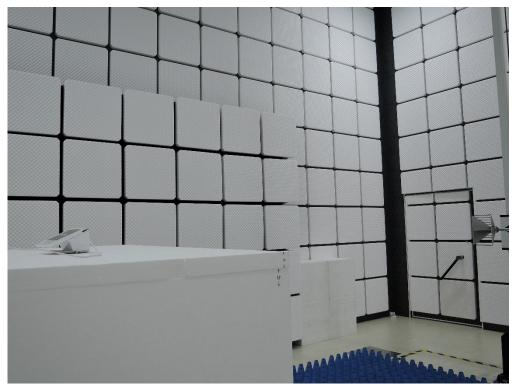
Radiated Emission Set up Photos (Front View)
