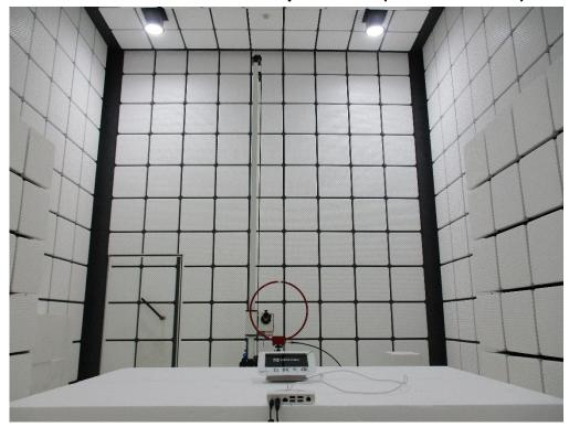
Radiated Emission Set up Photos (Below 1GHz)
