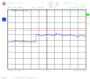
8.2.1.7 Out of Band Emissions at Antenna Terminals WCDMA B5, Middle channel, 836.4 MHz, 2 Hz to 1 GHz
