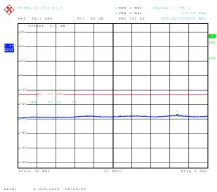
8.2.1.5 Out of Band Emissions at Antenna Terminals WCDMA B4, Middle channel, 1880 MHz, 1 GHz to 10 GHz
