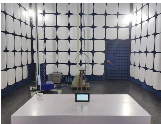
3. Radiated emission (9KHz-30MHz)
