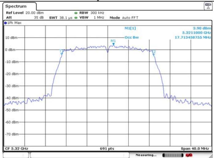
**U-NII-2A IEEE 802.11n HT20 5320MHz\_Ant 2****26dB Bandwidth****99% Occupied Bandwidth**
