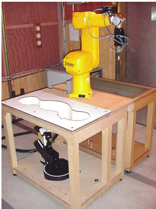
DASY4 SAR Measurement System with SAM phantom
