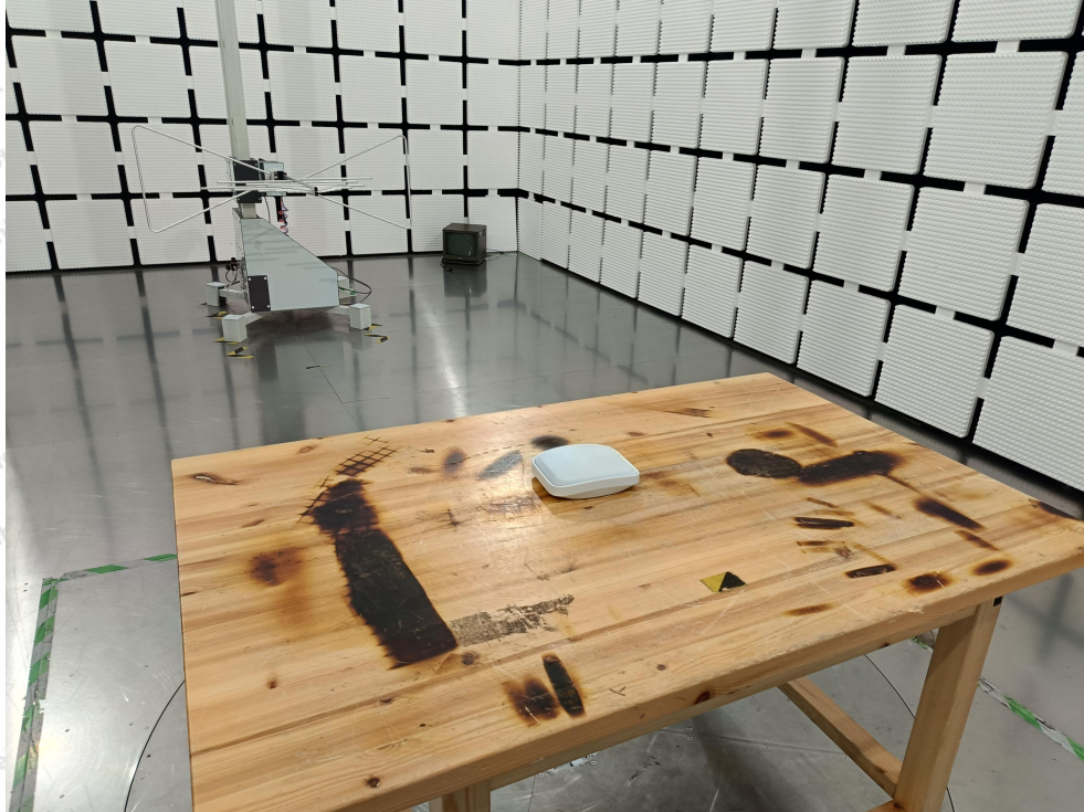
Photo of Radiation Emission Test
