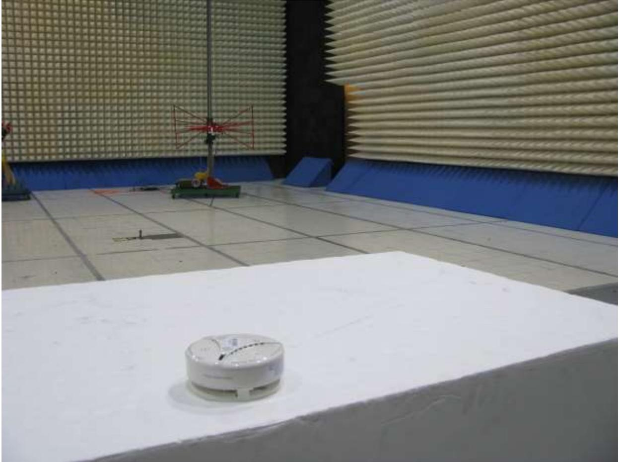
**Setup: Radiated Emissions (1Ghz to 18Ghz)**
