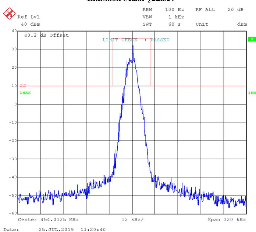
**4FSK,12.5 kHz, Low Power - Frequency 454.0125 MHz:****99% Occupied & 26 dB Bandwidth**
