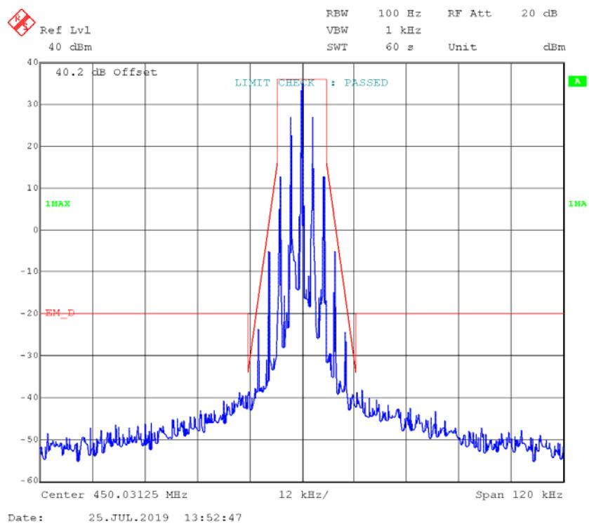
**FM,12.5kHz, Low Power – Frequency 450.03125 MHz:****99% Occupied& 26 dB Bandwidth**
