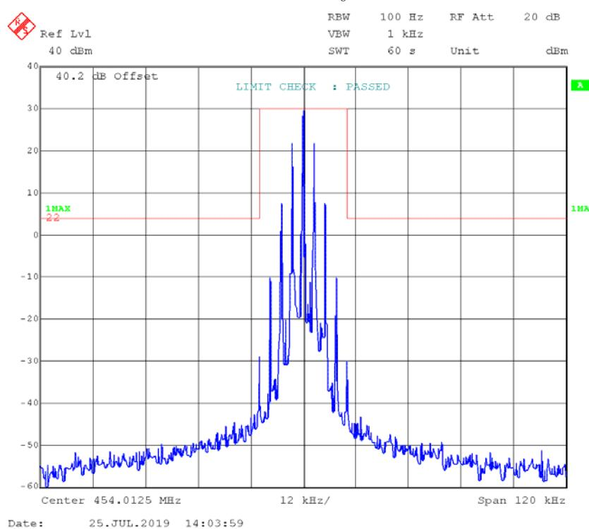
**FM,25kHz, High Power - Frequency 454.0125 MHz:****99% Occupied & 26 dB Bandwidth**
