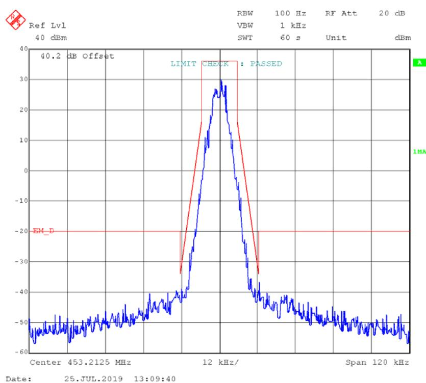
**4FSK,12.5kHz, Low Power - Frequency 453.2125 MHz:****99% Occupied& 26 dB Bandwidth**
