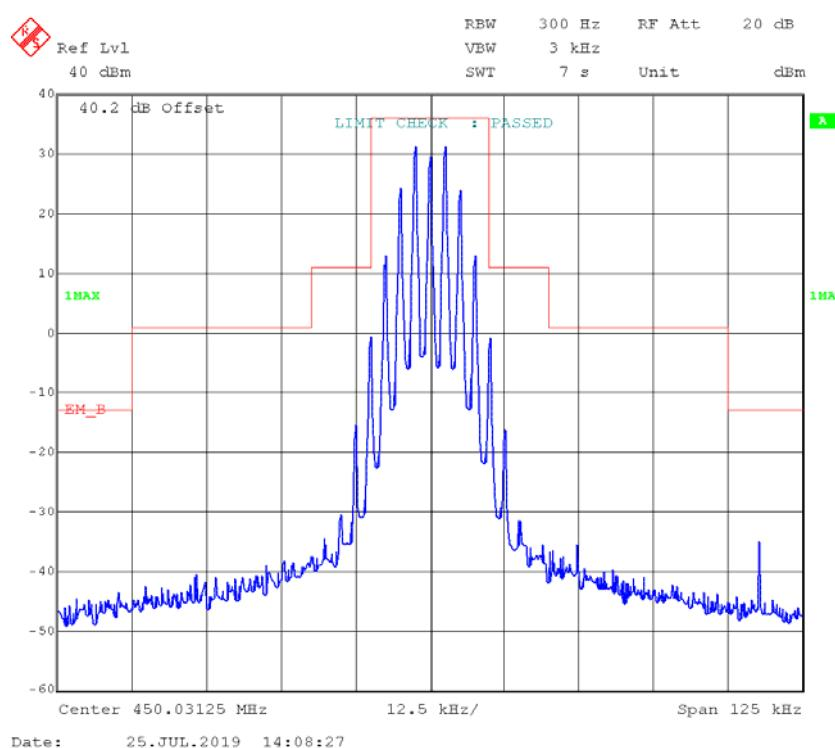
**FM, 25 kHz, Low Power – Frequency 450.03125 MHz:****99% Occupied & 26 dB Bandwidth**
