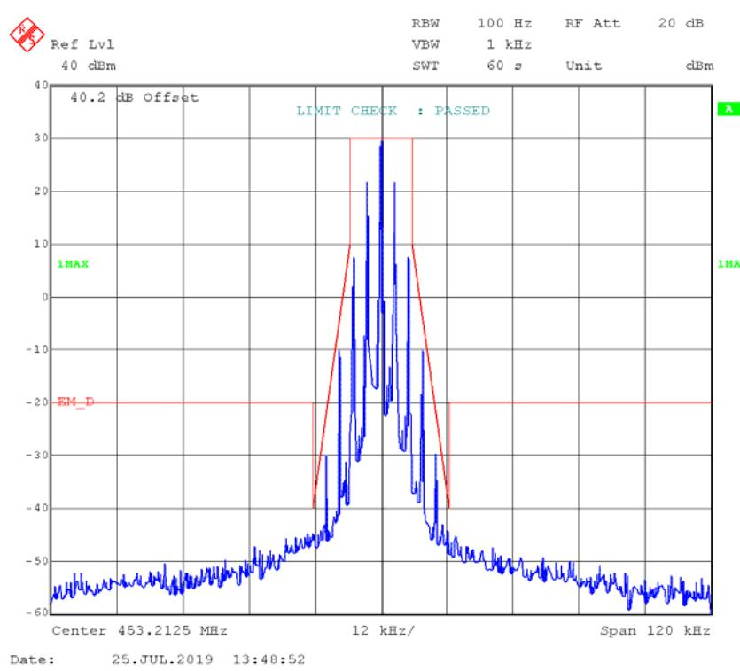
**4FSK,12.5kHz, High Power - Frequency 453.2125 MHz:****99% Occupied & 26 dB Bandwidth**
