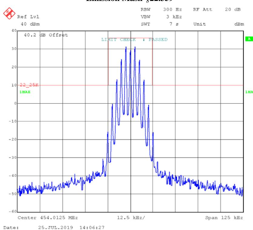
**FM, 25 kHz, Low Power – Frequency 454.0125 MHz:****99% Occupied & 26 dB Bandwidth**
