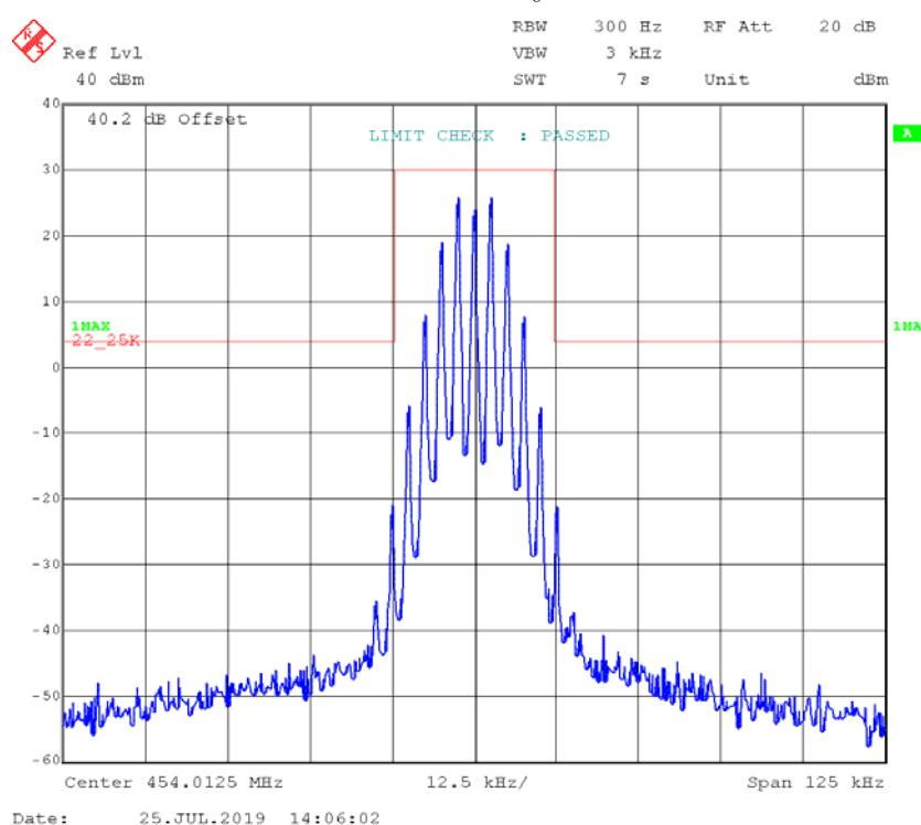
**4FSK,12.5 kHz, High Power - Frequency 454.0125 MHz:****99% Occupied & 26 dB Bandwidth**
