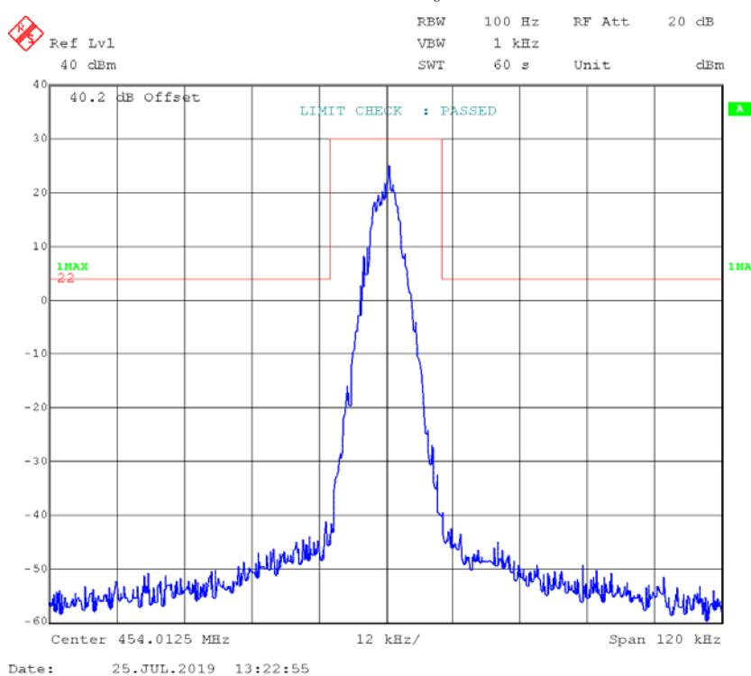
**Part 74****FM,12.5kHz, High Power - Frequency 450.03125 MHz:****99% Occupied& 26 dB Bandwidth**
