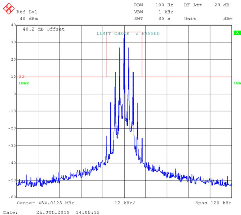
**FM,12.5kHz, Low Power – Frequency 454.0125 MHz:****99% Occupied & 26 dB Bandwidth**
