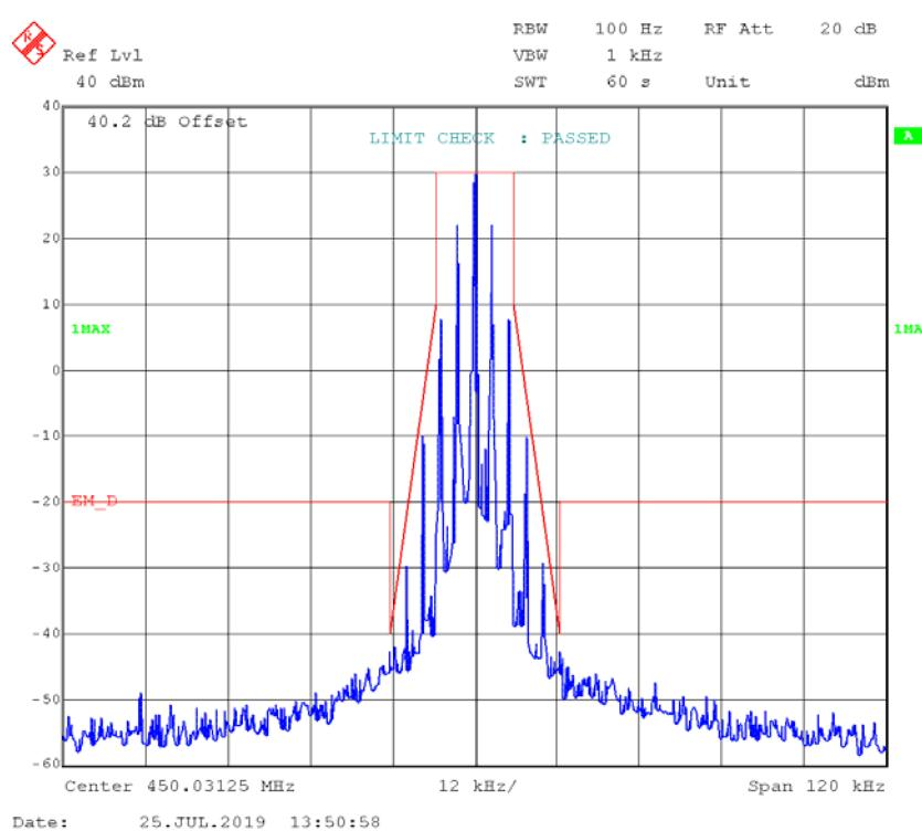
**FM,25kHz, High Power - Frequency 450.03125 MHz:****99% Occupied & 26 dB Bandwidth**
