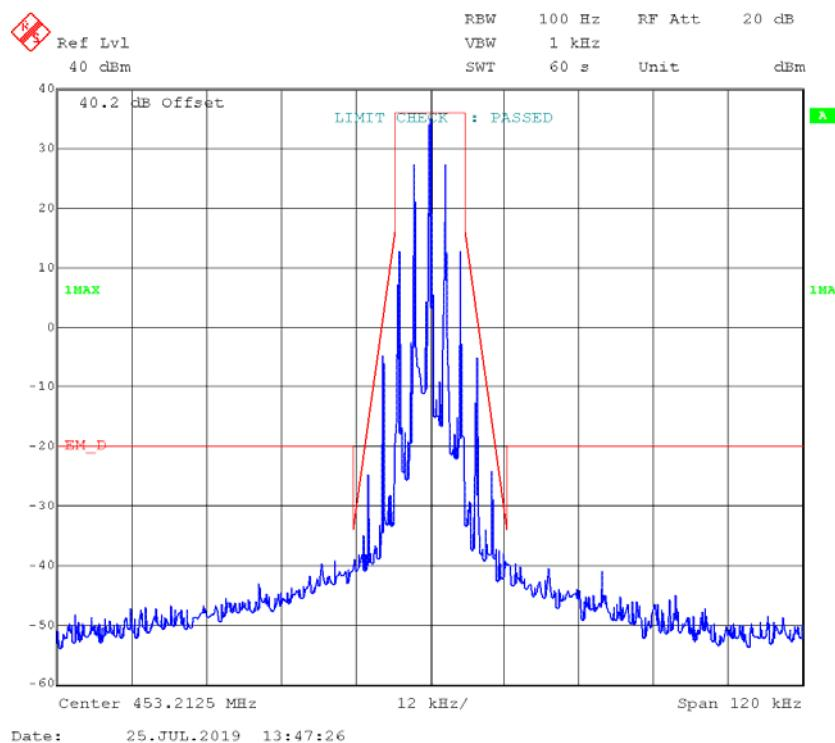
**FM,12.5kHz, Low Power - Frequency 453.2125 MHz:****99% Occupied & 26 dB Bandwidth**
