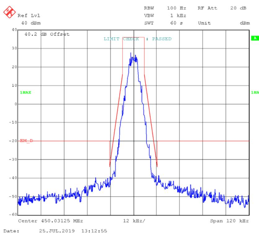
**4FSK,12.5 kHz, Low Power - Frequency 450.03125 MHz:****99% Occupied & 26 dB Bandwidth**
