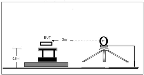
(B) Radiated Emission Test-Up Frequency 30MHz~1GHz
