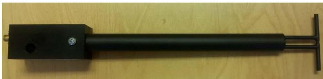
Figure 1 – MVG COMOSAR Validation Dipole
