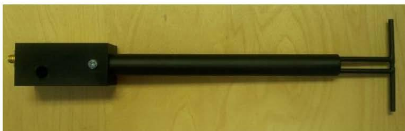
Figure 1 – MVG COMOSAR Validation Dipole
