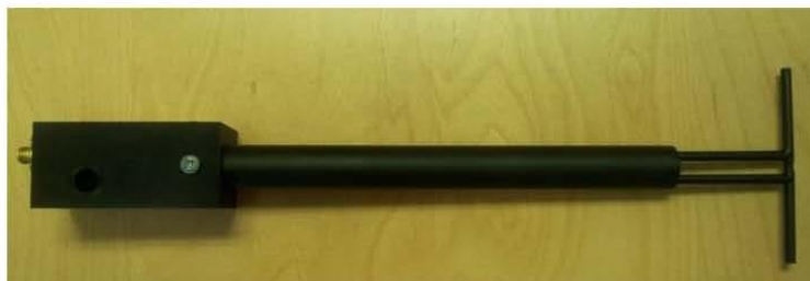
Figure 1 – MVG COMOSAR Validation Dipole
