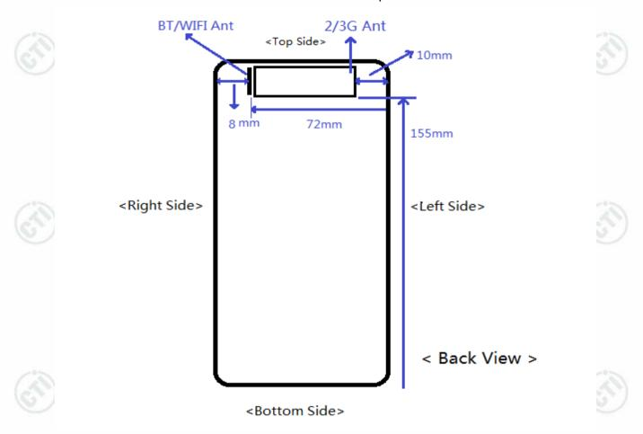
The SAR measurement positions of each side are as below:
