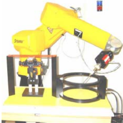
Figure 4: T-Coil set up with HAC Test Arch with Helmholtz Coil (AMCC)
