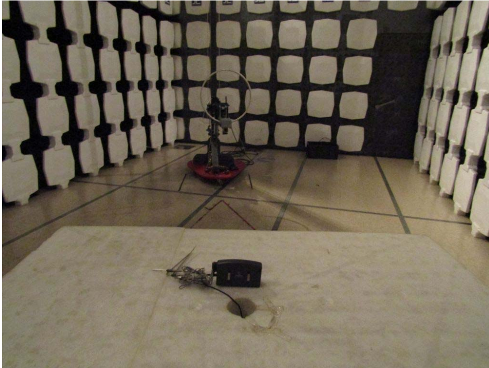
Measurement of Radiated Emission Test Set Up
