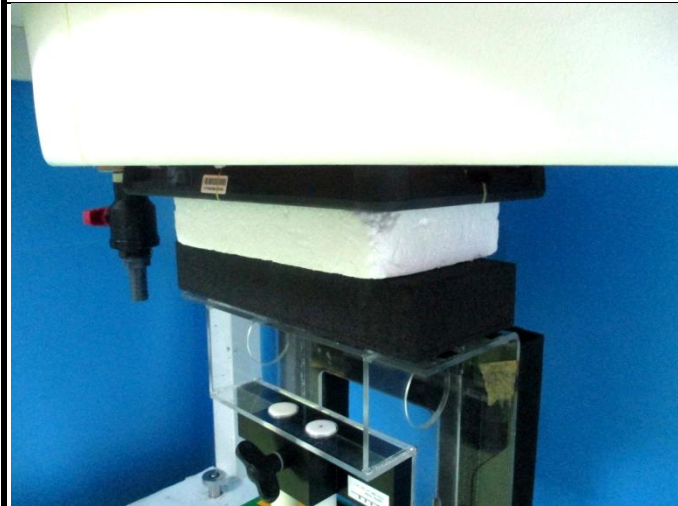
Rear Face of EUT with 0 mm Gap
