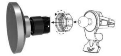
.Unscrew the nut .Place the nut around ball head, insert into socket .Tighten nut clockwise
