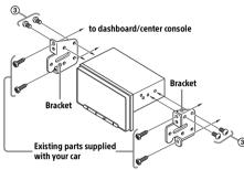
When mounting this unit to the preinstalled brackets of your car, use the mounting screws ③ in the appropriate screw holes based on your car: T for TOYOTA and N for NISSAN.
