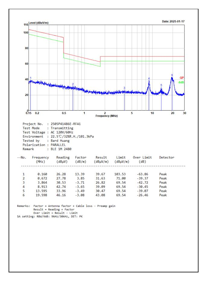
For radiated emissions below 30MHz, there were no emissions found within 20dB of limit.
