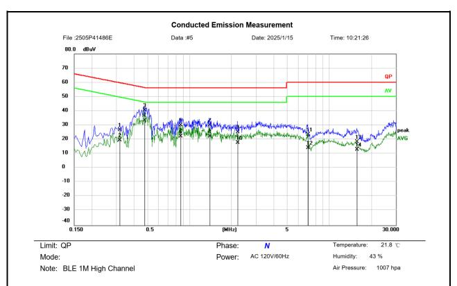
Receiver Setting: 0.15~30MHz: Pre-scan: RBW: 9kHz, DET: PK/AV; Final measure: RBW: 9kHz, DET: QP/AV
