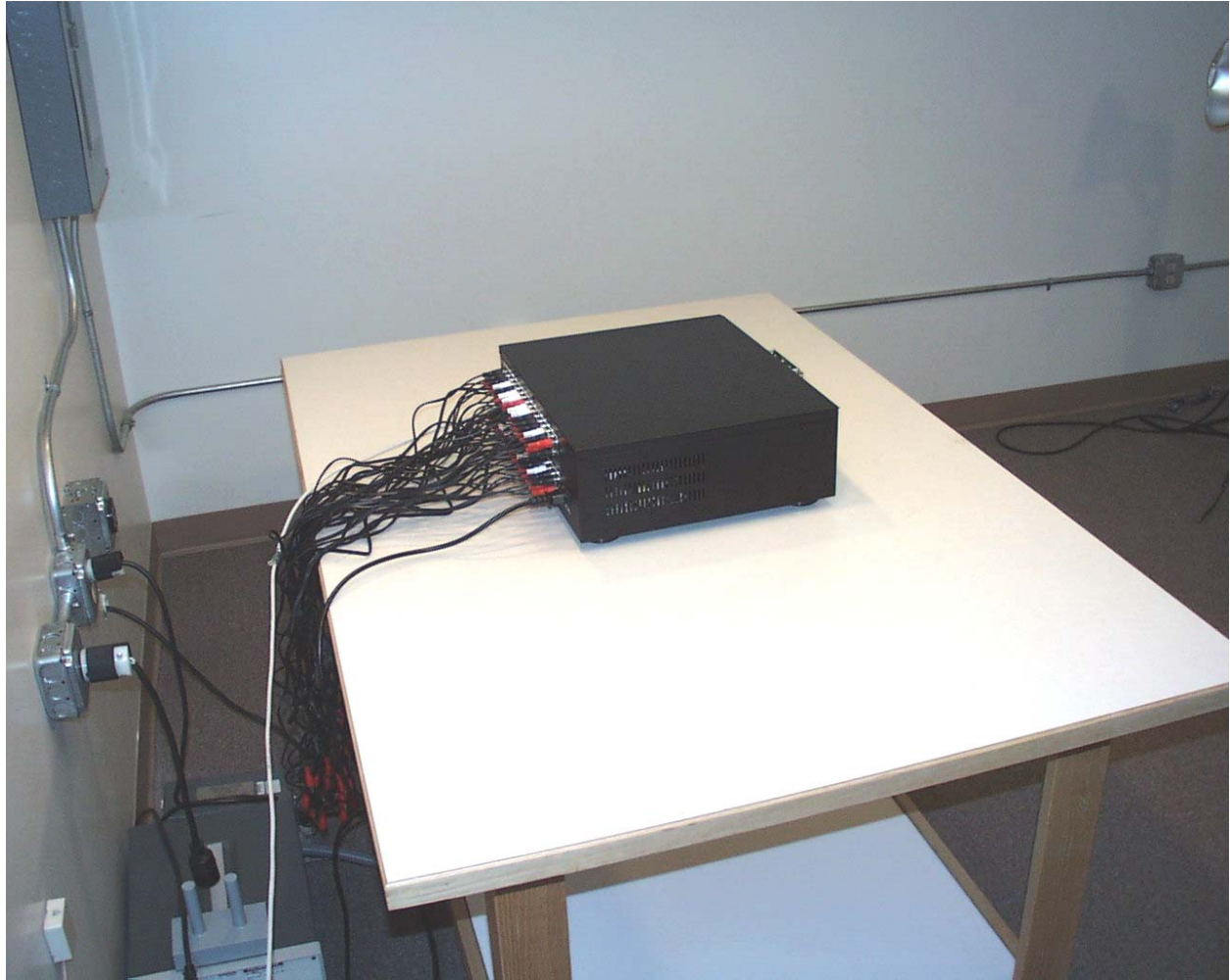
Photograph 4 - Back View Conducted Disturbance Worst Case Configuration
