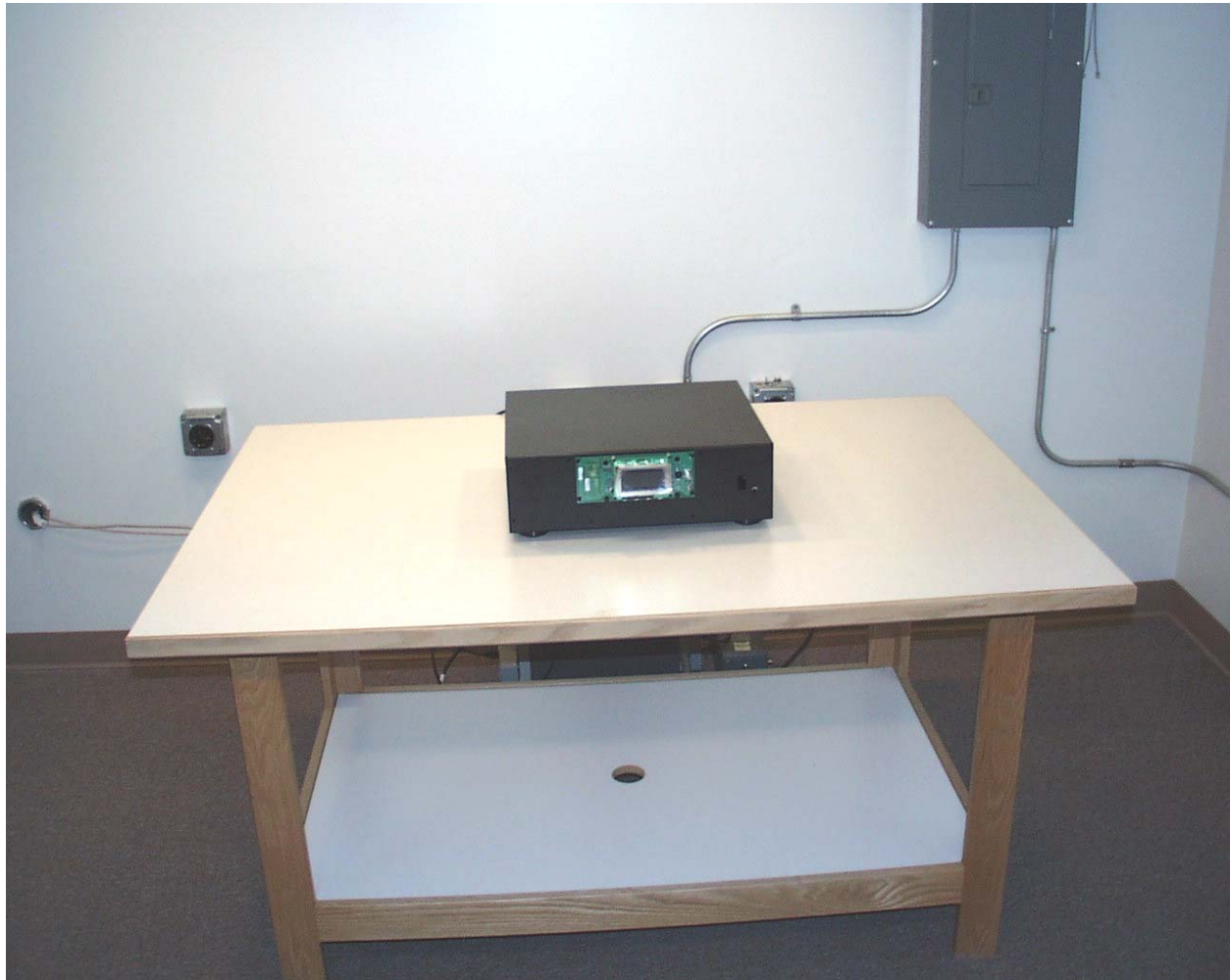
Photograph 3 - Front View Conducted Disturbance Worst Case Configuration
