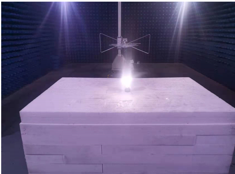
Photo of Radiated Emission Measurement (Above 1G)
