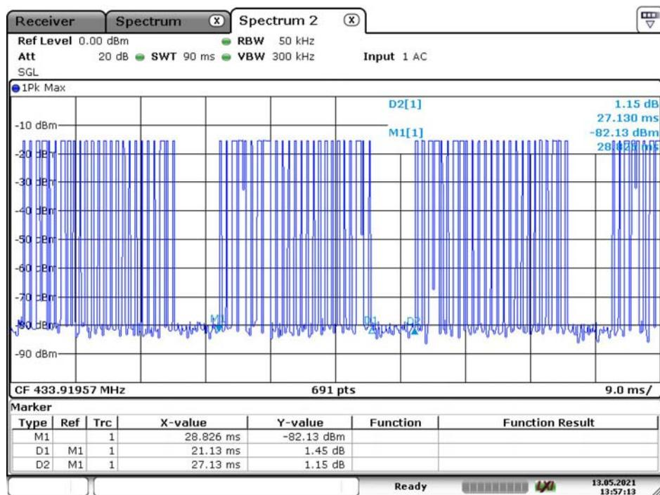
$T_{on1} = 5\text{ms}, T_{on2} = 20\text{ms}$
