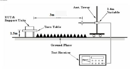
The radiated emission tests were performed in the 3 meters chamber test site, using the setup accordance with the ANSI C63.10-2013. The specification used was the FCC 15.209, FCC 15.407 and RSS-247, RSS-Gen limits.
