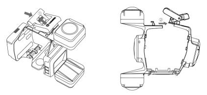
**Step 2:** As shown below, lock the mounting bracket's connection buckle onto the bottom of the drone.
