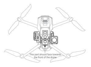
**Step 3:** Lock the Lock Lever well and ensure that the yellow mark of the Lock Lever is not showing.
