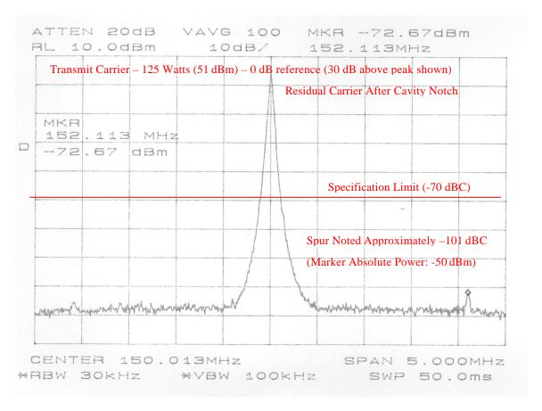
Note: The absolute power of the spur was verified using the substitution method. A signal generator was fed into the same notch test setup as the transmitter. The power level of a 152.113 MHz carrier was adjusted until equivalent power level as the spur shown above (–72.67 dBm) was observed at the spectrum analyzer. This absolute power level was then compared to the power level of the transmitter to obtain the spur power level referenced to the carrier power.
