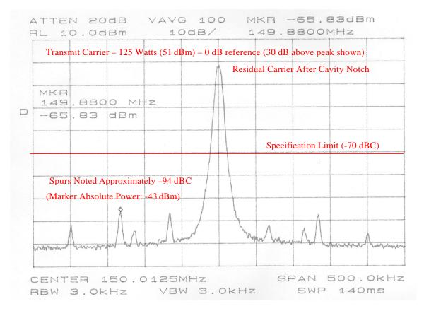
Note: The absolute power of the spur was verified using the substitution method. A signal generator was fed into the same notch test setup as the transmitter. The power level of a 149.88 MHz carrier was adjusted until equivalent power level as the spur shown above (–65.83 dBm) was observed at the spectrum analyzer. This absolute power level was then compared to the power level of the transmitter to obtain the spur power level referenced to the carrier power.
