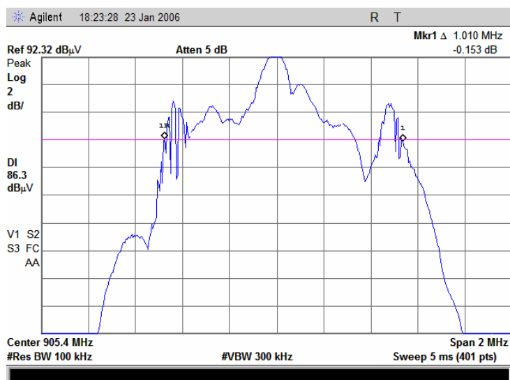
Plot 7.1.1 The 6 dB bandwidth test result at low frequency, PSK modulation
