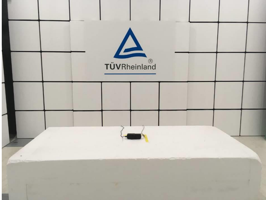
Photograph 2: Test Setup for Spurious Emissions (Front View 2)
