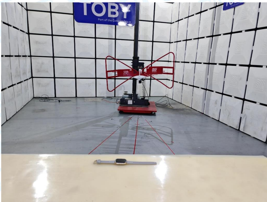
Photo of Setup for Radiated Emission (30MHz~1GHz)
