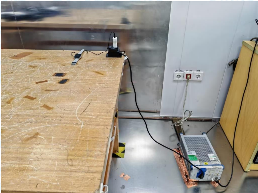
Photo of Setup for Radiated Emission (30MHz~1GHz)
