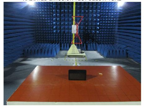
RADIATED EMISSION TEST ABOVE 1GHZ
