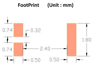
• 2<sup>nd</sup> Layout Dimensions in Clearance area(Size=8.0\*3.0mm)
