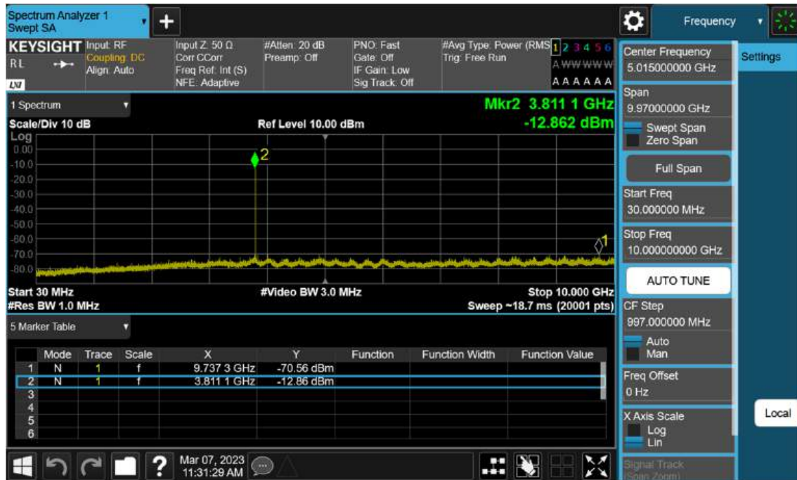
Sub6 n77(78). Conducted Spurious Plot_1 (656000ch_60 MHz_BPSK)
