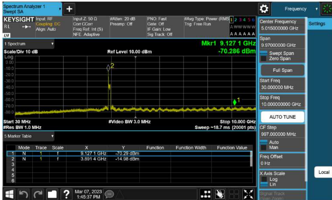
Sub6 n77(78). Conducted Spurious Plot_1 (662332ch_90 MHz_BPSK)
