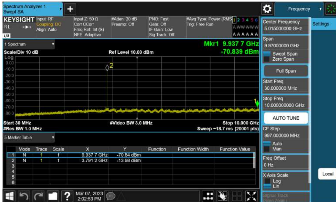
Sub6 n77(78). Conducted Spurious Plot_1 (656000ch_100 MHz_BPSK)
