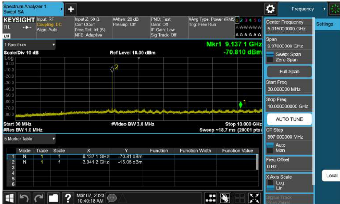
Sub6 n77(78). Conducted Spurious Plot_1 (664000ch_40 MHz_BPSK)
