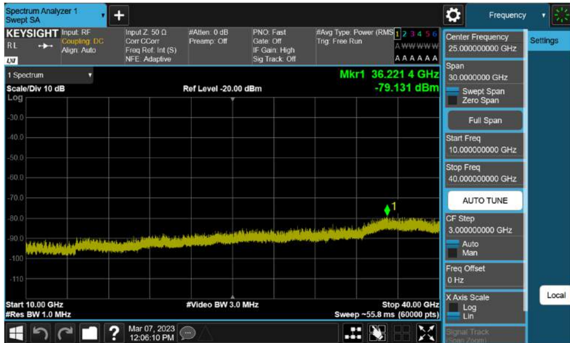
Sub6 n77(78). Conducted Spurious Plot_2 (656000ch_80 MHz_BPSK)
