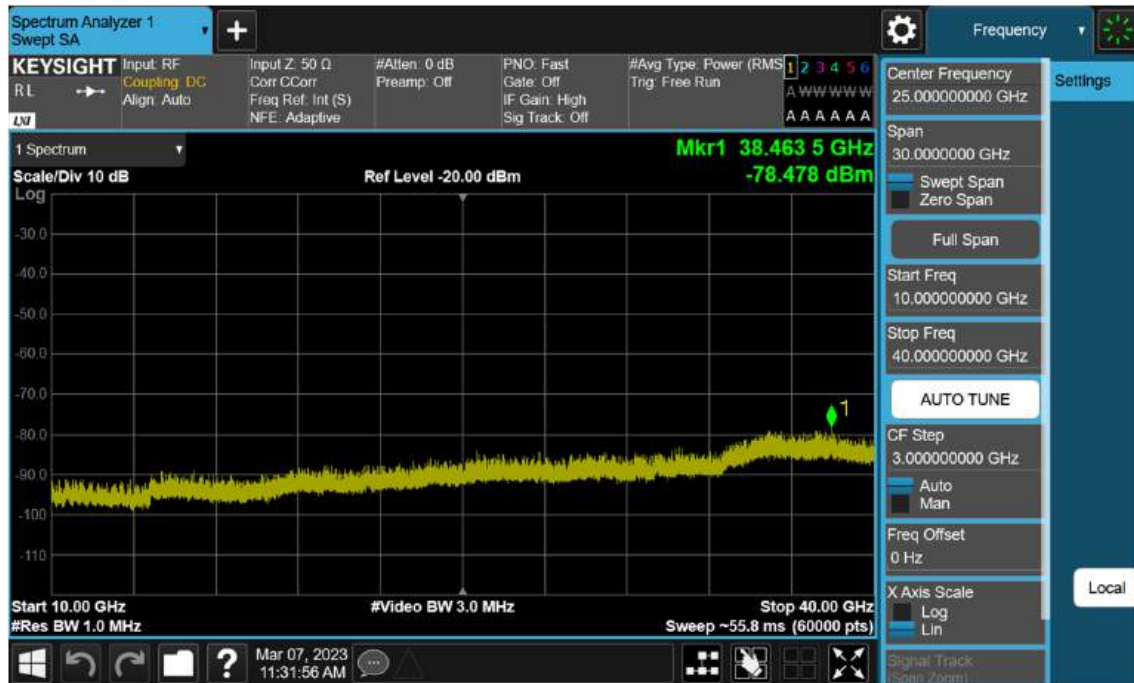
Sub6 n77(78). Conducted Spurious Plot_2 (656000ch_60 MHz_BPSK)
