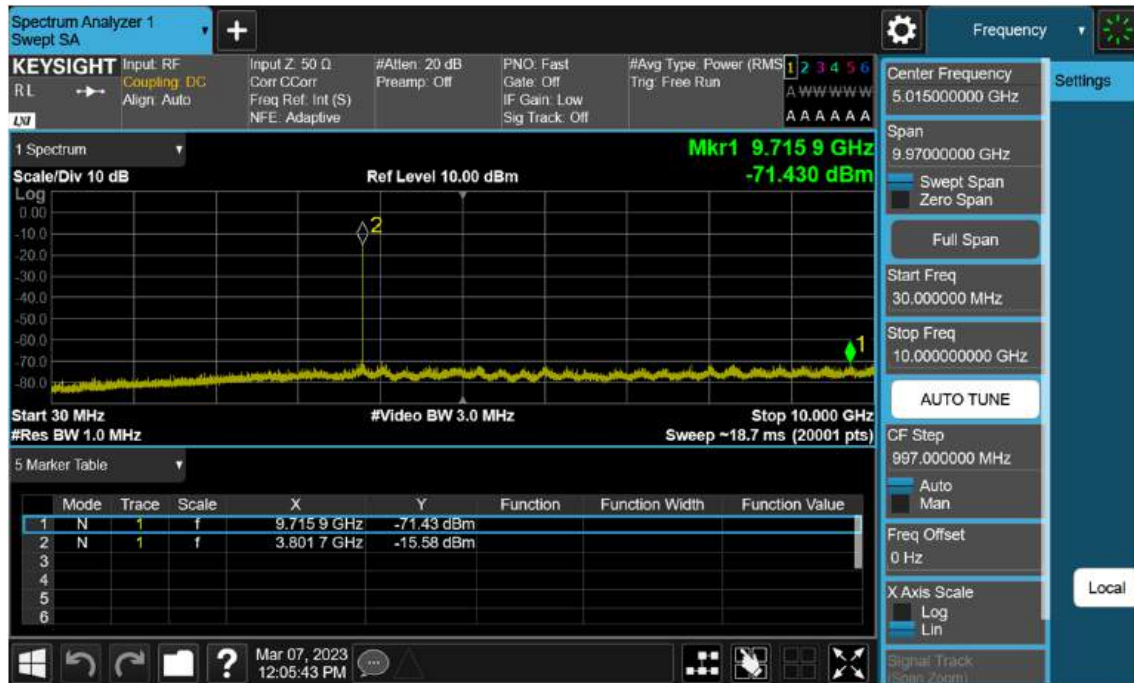
Sub6 n77(78). Conducted Spurious Plot_1 (656000ch_80 MHz_BPSK)
