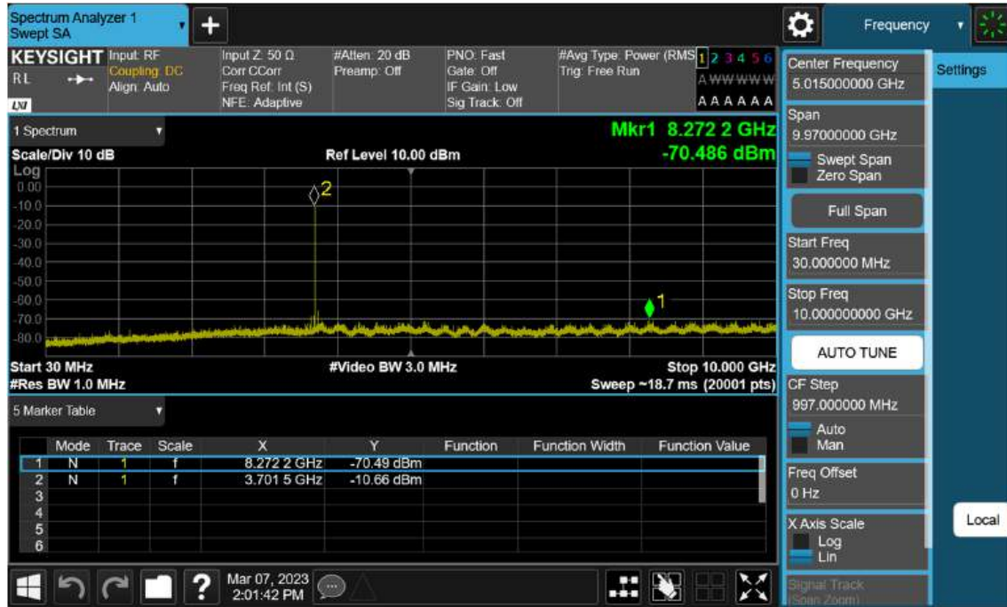
Sub6 n77(78). Conducted Spurious Plot_1 (650000ch_100 MHz_BPSK)
