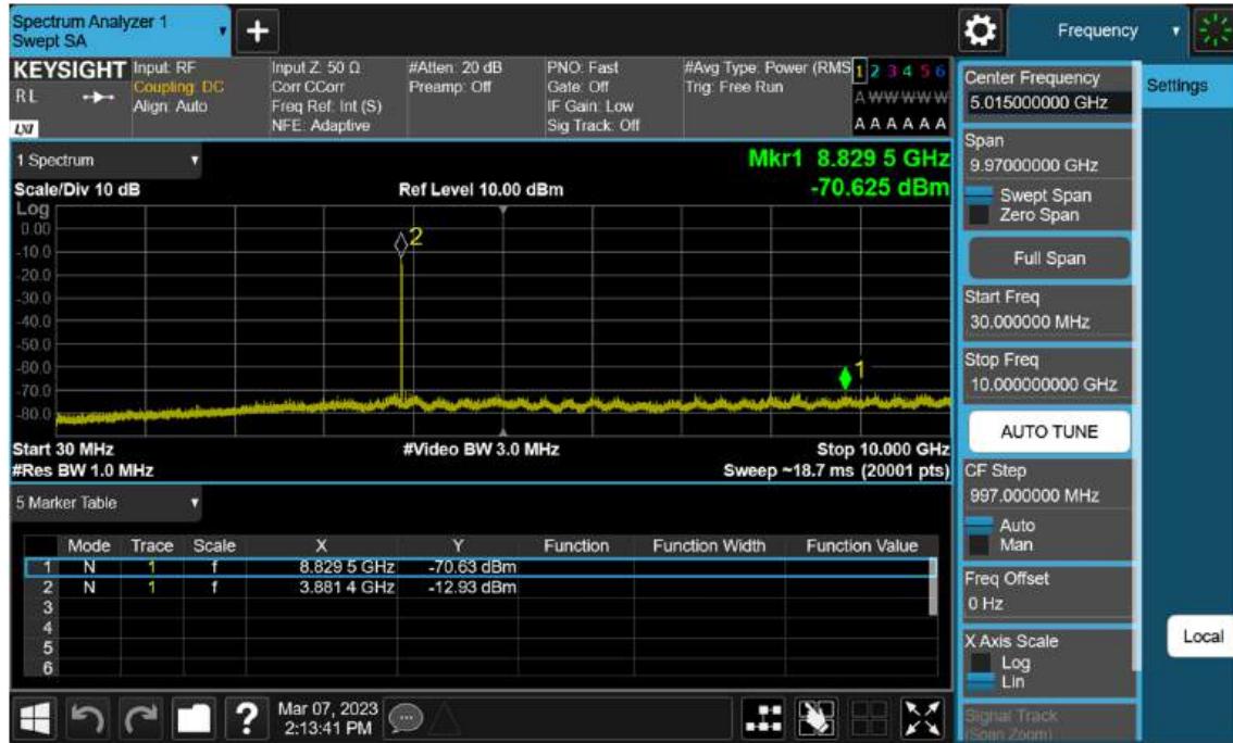
Sub6 n77(78). Conducted Spurious Plot_1 (662000ch_100 MHz_BPSK)
