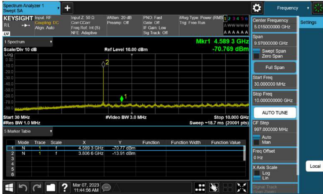
Sub6 n77(78). Conducted Spurious Plot_1 (656000ch_70 MHz_BPSK)
