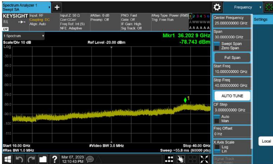
Sub6 n77(78). Conducted Spurious Plot_2 (662666ch_80 MHz_BPSK)
