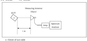
Distance Factor:  $20 \times \log (4.0 \text{ m}^*/3.0 \text{ m}) = 2.5 \text{ dB}$ \* Test Distance: (3 + Test Volume /2) - r = 4.0 m
