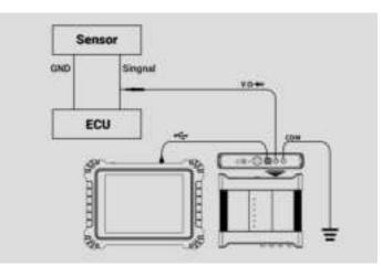
Figure 1-16 Sample Arbitrary Waveform Connection Diagram
