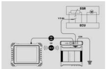
Figure 1-11 Sample DC Voltage Connection Diagram
