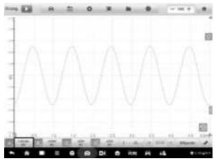
Figure 1-52 Sample Amplitude Setting Screen (DC 1.0V/div)
