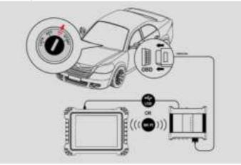
Figure 1-60 Sample DLC Connection Diagram
