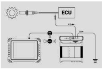
Figure 1-13 Sample Square Wave Connection Diagram
