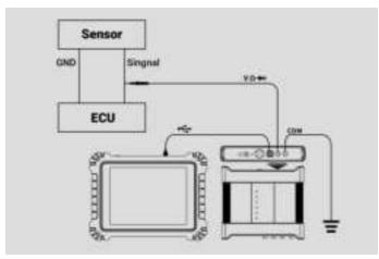
Figure 1-15 Sample Triangle Waveform Connection Diagram
