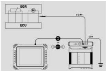
Figure 1-12 Sample Actuator Drive Connection Diagram
