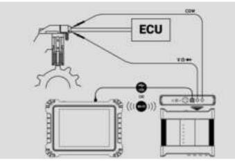
Figure 1-14 Sample Square Wave (X+Y) Connection Diagram
