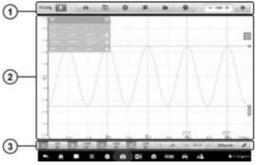
Figure 1-6 Sample Oscilloscope Menu Screen
